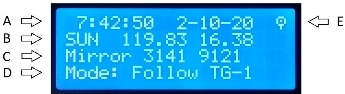
Use the remote control slider position 3 to check if the motors turn the right direction and if the absolute value (C) counts the right way. If the encoder counts the wrong direction the motor will not stop running, press Stop and cross the AB signal.
