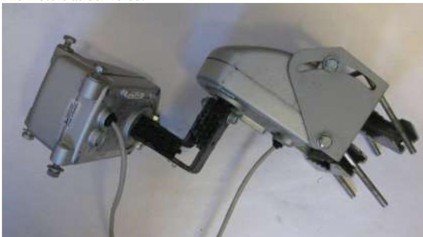
Left the vertical motor and right the horizontal.
