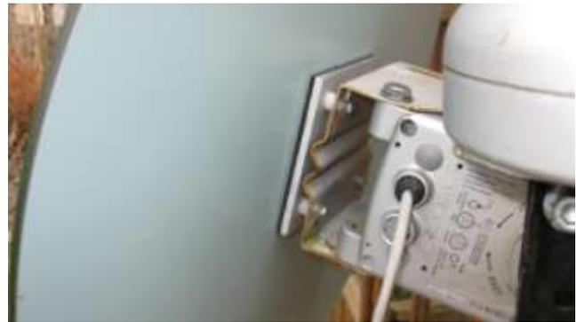
Another way of mounting. A sheet of aluminium with foam 100x100x4mm tapped with 5mm thread.
